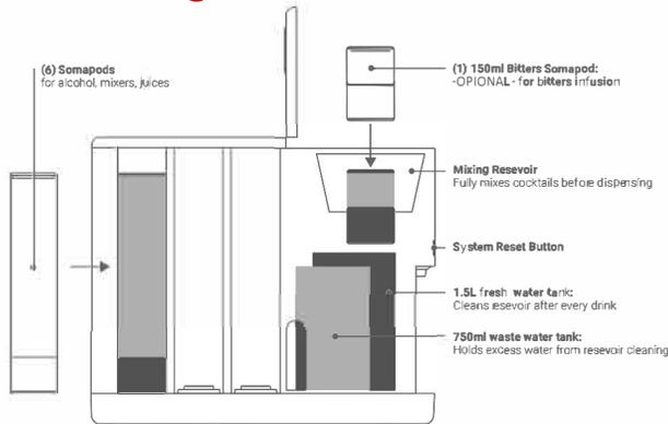
Fill Somabar's fresh water tank with water and then plug Somabar into a standard wall outlet.
